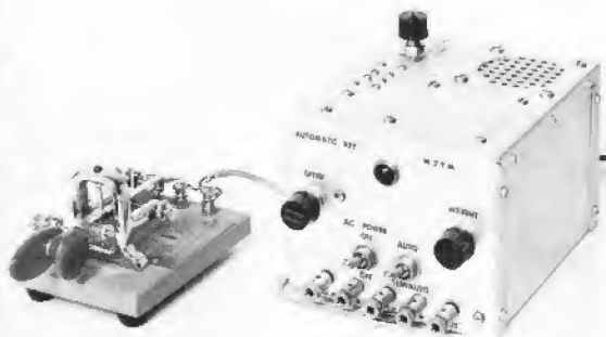
W2YM's transistorized keyer can be operated either as a semi-automatic "bug" key or fully automatic key. Instrument is shown here with a Vibroplex "Vibro-Keyer" connected to it. Standard hand key can be connected to two binding posts at left.
